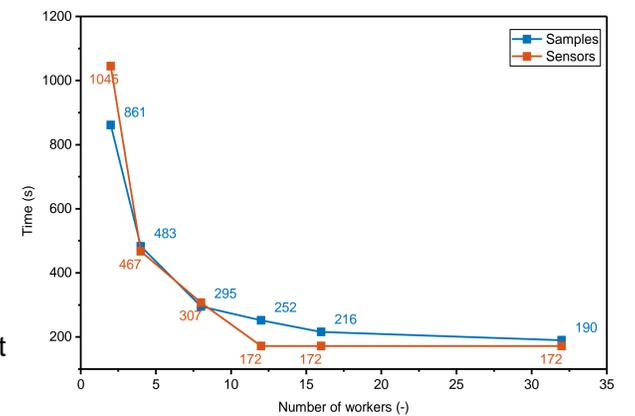
Figure 4: Processing time for an individual machine of the proposed system with different HPC configuration..
