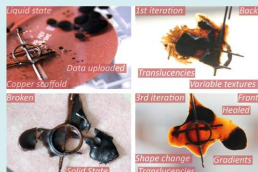
Preliminary ferro-wax structure that can be melted and reprogrammed to change shape and self-heal via a multi-stimuli system.
