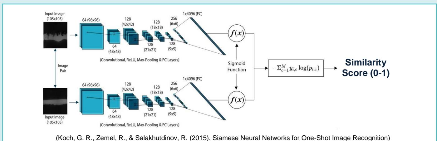
The model architecture utilised in this study comprises two identical 13-Layer Convolutional Subnetworks, first developed by (Koch et al., 2015). By comparing similarity to the nominal (non-defective) state rather than assigning images to discrete classes, it is possible to detect new (unseen) defect types without retraining the network.
